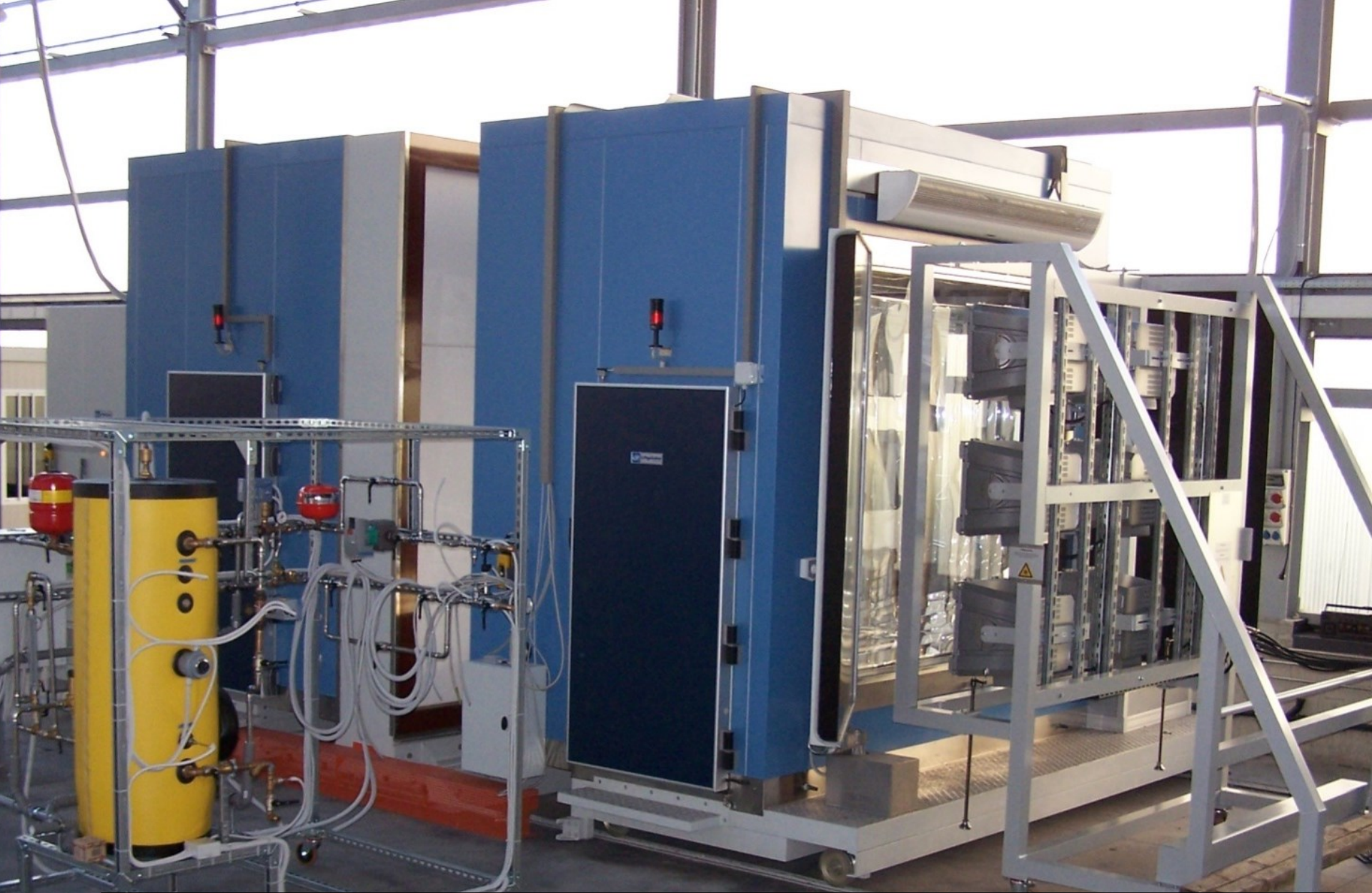
Test facility (double guarded hot box) for testing thermal properties of building envelopes, passive and solar active (artificial sun)
