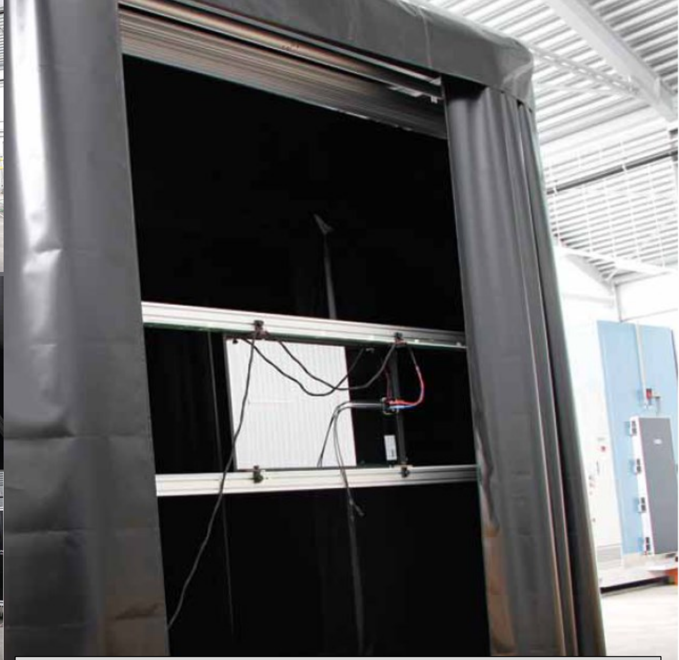
PV Laboratory - Indoor test facility for PV module characterization according to IEC standards
